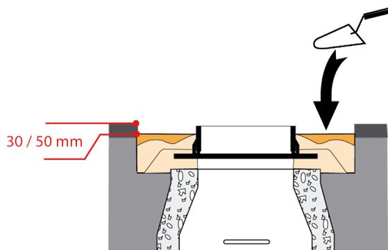
**9** Use a float or trowel to level off the product, leaving 3 to 5 cm for the later laying of the asphalt course.
