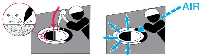
**2** Check the condition of the manhole opening or groove, removing any debris, loose particles or dirt (oil, grease, etc.).
